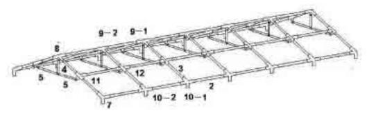
Fastening the roof by using turnbuckle set(18) which is diagonally across through each two section as below .
